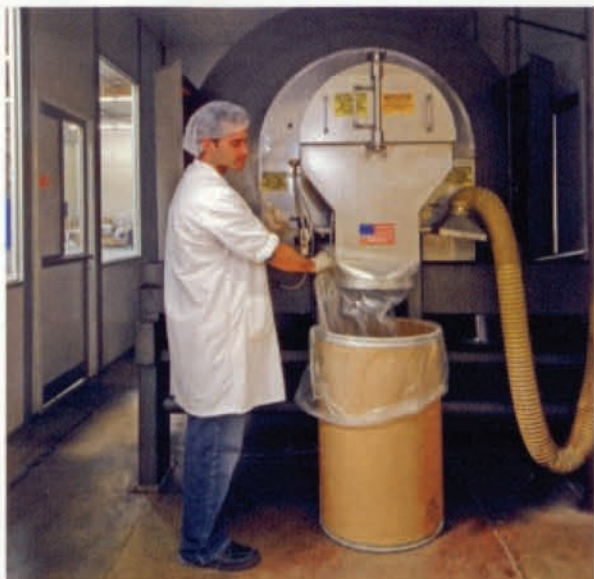
Internal mixing flights elevate the material which is discharged through a plug gate valve into plastic-lined drums.
