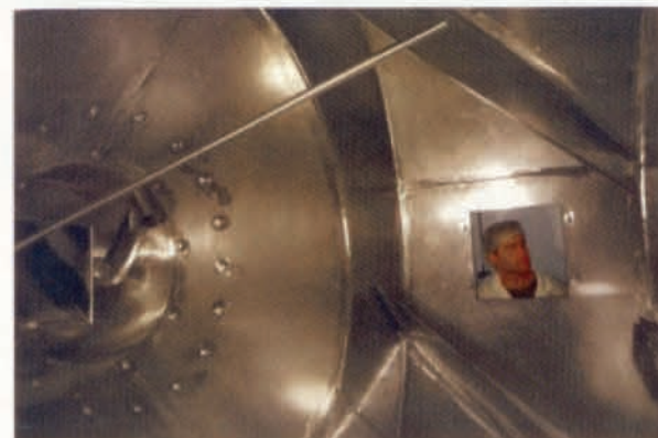
Rotating drum with proprietary mixing flights achieves total batch uniformity in less than three minutes.
